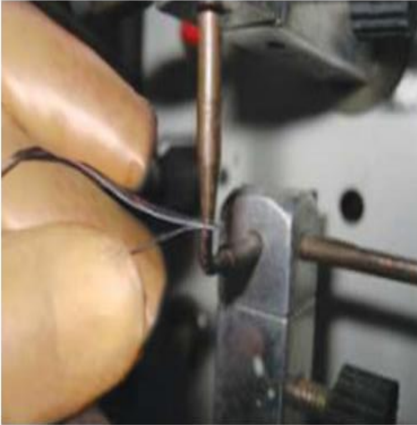
Fig. 35.2A: Initial spot weld
